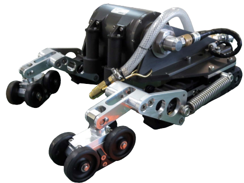
Standard and modified Magg™ miniature magnetic inspection crawlers
