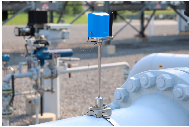
Figure 1: Ultra-High-Temp attached with a band clamp.
